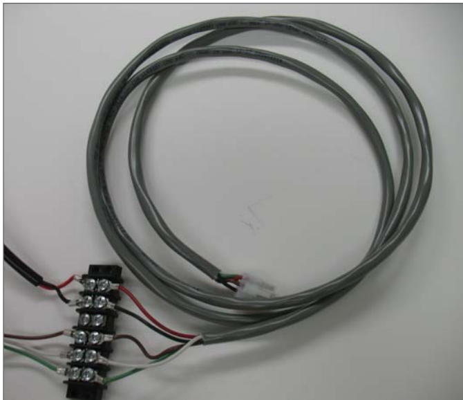
Fig. 4 Example of an LED CoveWash 6 Feet Power Cable 504488-06
