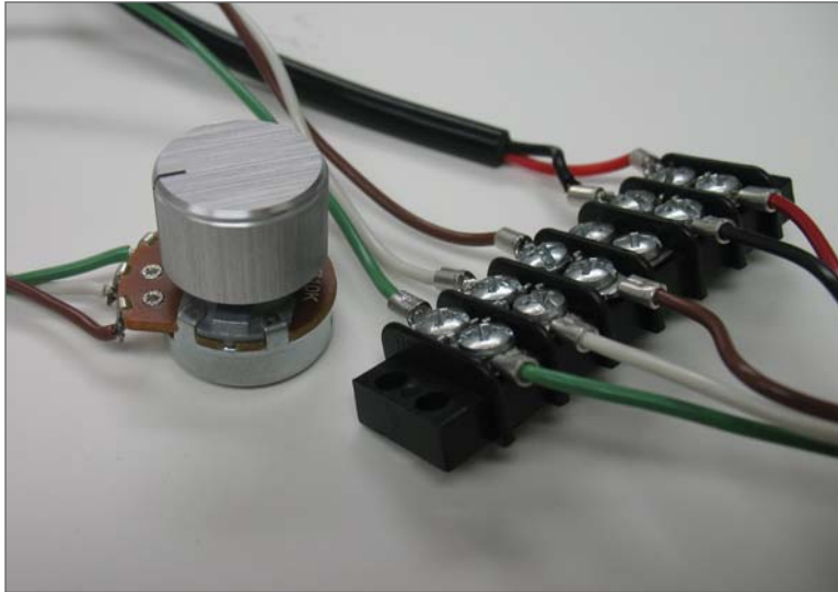
Fig. 5 Manual Dimming Control wired with a 6-Position Terminal Block, a 10K Ohm Potentiometer , and a Knob Left Cable is the output of the 24 VDC Class 2 Power Supply Right Cable is DDP Power Cable 504488-06
