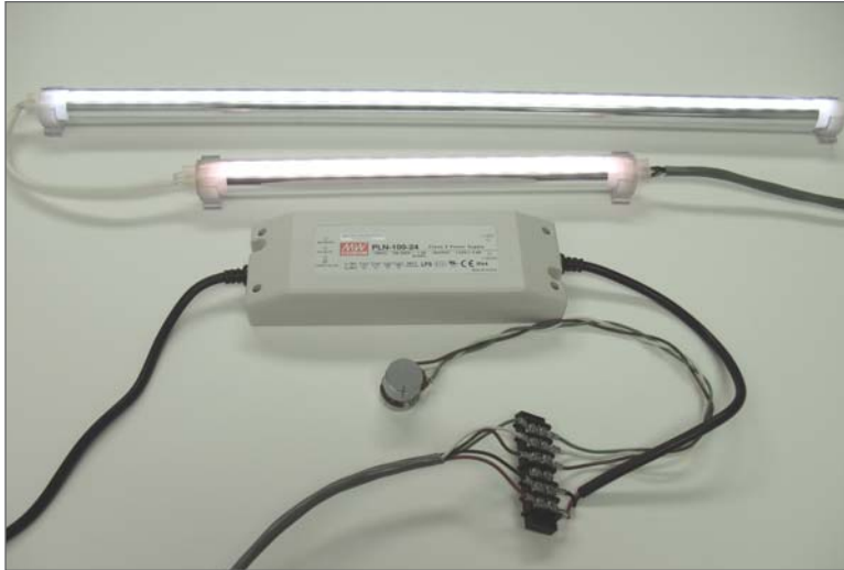
Fig. 1 Example of LED CoveWash units in Cascade Mode powered by a 100-Watts 24 VDC Class 2 Power Supply with Dimming Connections
